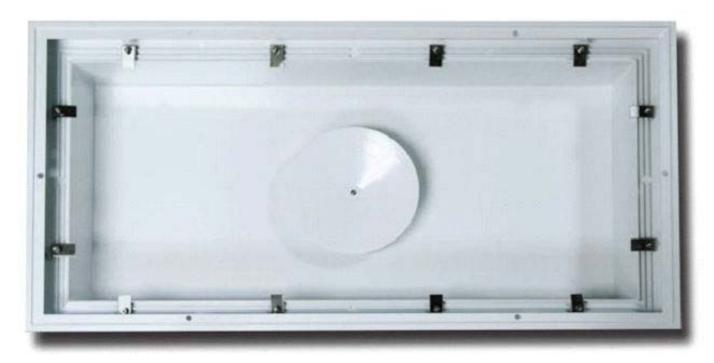
6. Turn clips to be parallel to diffuser frame to allow filter to be positioned without obstruction.
