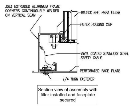
10. Precision Air Products recommends that the filters be in place for at least 12 hours prior to any type of clean room certification testing which may be required.
