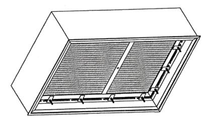
Figure 4A. Installed filter with retaining clips in place, putting pressure against filter's gasket or gel seal.
