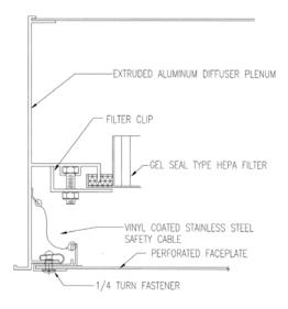
Figure 4B: Section view of installed filter with gasket seal filter.
