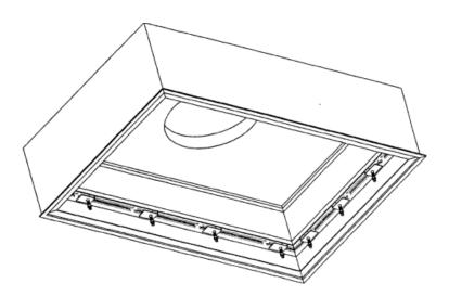
Figure 3. Retaining clip positioning prior to filter installation with "knife edge" of diffuser ready to mate with filter's gasket or gel seal.
