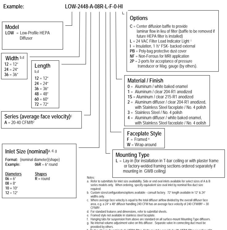
h. Codes shown do not include HEPA filter. Units must be provided with HEPA filter or option "C" in order to achieve cataloged performance. Specify filters according to next page (Form # 4-308).
